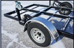
The image to the right illustrates the hitch assy on the fish house frames. It is a crank down tongue. While the hitch is being cranked down, the receiver stays in the air and the rest of the frame lowers to the ice. This tongue is equipped with a heavy duty crank jack and a 2 inch coupler for a 2 inch ball.
